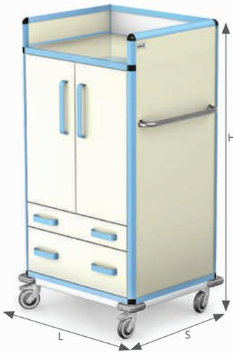
Elements of **WMW series trolleys** are made of: **frame** of closed aluminium profiles and ABS connectors, anodized or powder coated in the colour according to RAL palette TECH-MED sample-card **filling** of chipboard laminated on both sides **top** of chipboard, enclosed on three sides **steel base**, powder coated; equipped with castors of 100 mm diameter, including two with a block-ade, base with buffers at the corners
